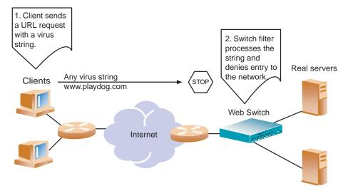
Figure 15-9 Configuring Layer 7 Deny Filter
